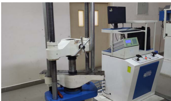
Fig. 1: Experimental setup of the compaction die
